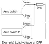
(Solid state) When two auto switches are connected in parallel, malfunction may occur because the load voltage will increase when in the OFF state.
