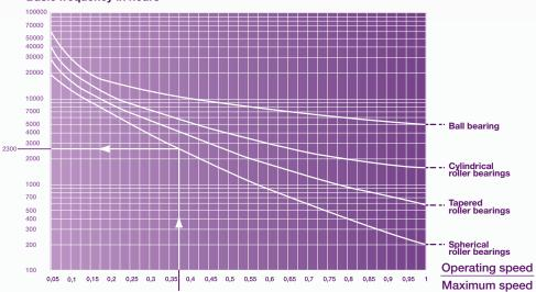
The basic frequency (Fb) of relubrication depends on the type of bearing and the ratio of operating speed to the maximum speed indicated in the bearing characteristics.
