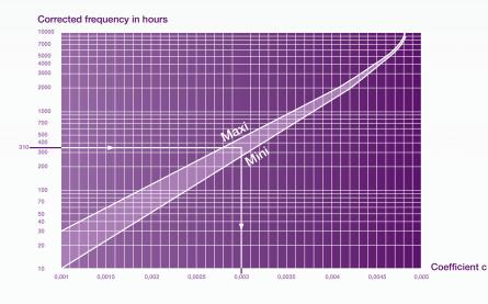
This corrected frequency can be used to determine the weight of grease to be added, depending on:
