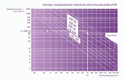
➤ Then calculate the viscosity of the lubricant to be selected on the basis of the service temperature of the bearing.
